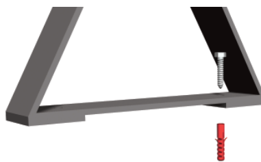
Vandalensichere Verschraubung Vandal-safe screw-fitting
