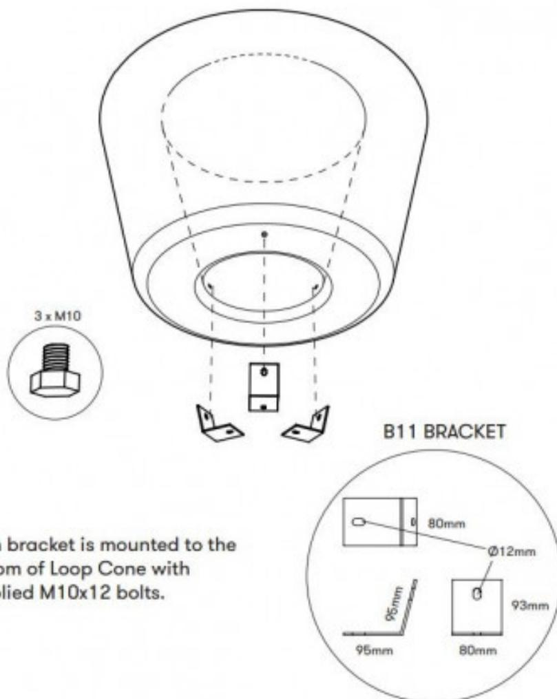
Each bracket is mounted to the bottom of Loop Cone with supplied M10x12 bolts.
