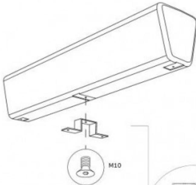
The bracket is mounted onto the bottom of Loop Line with supplied M10x16 unbrako bolt.
